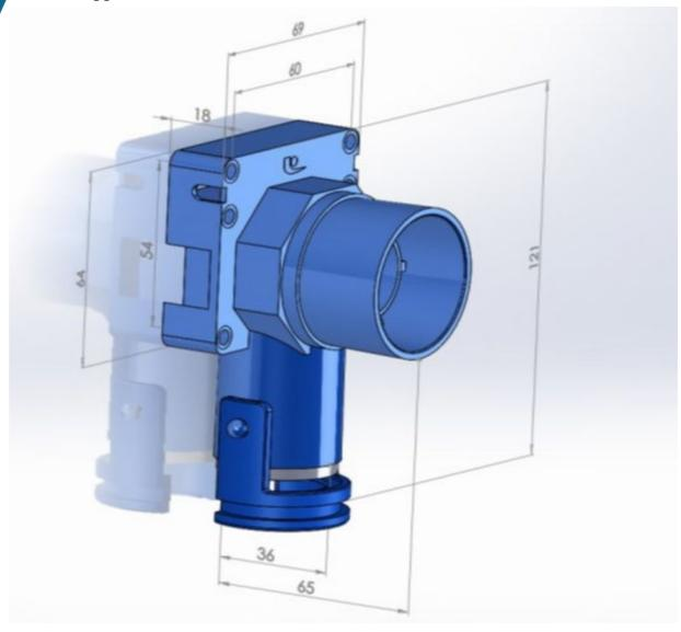
The thickness of the frame is 36mm from the top of the housing pipe, which is the minimum thickness of the wall frame.
